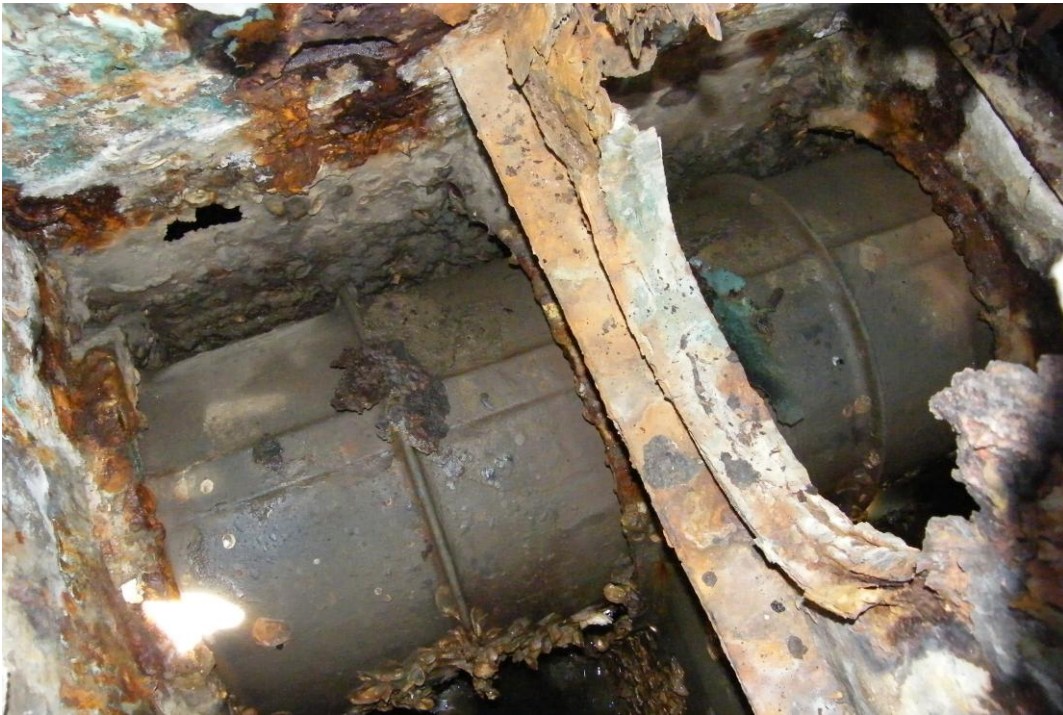
Wasted structure around bronze torpedo tube.
