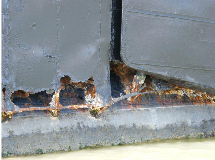
Detail of forward plane to starboard, showing wasted superstructure deck framing and face plating.
