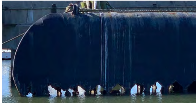
Down by the head bow structure surrounding forward torpedo tubes 2019.
