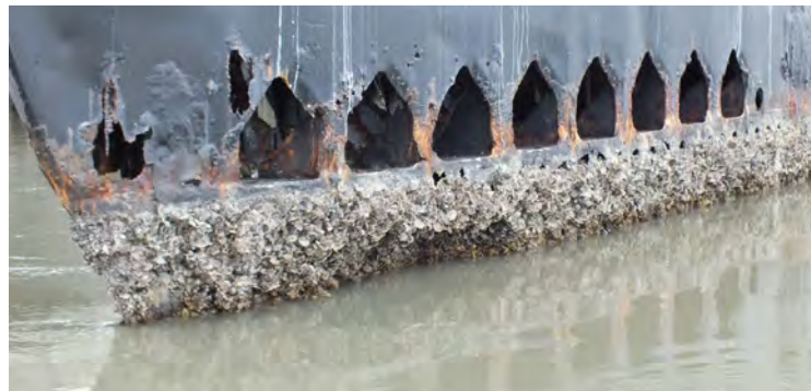
Bow structure surrounding forward torpedo tubes, 2012. Notice heavy beard of shellfish growth on bottom necessitating UHP wash of hull bottom.
